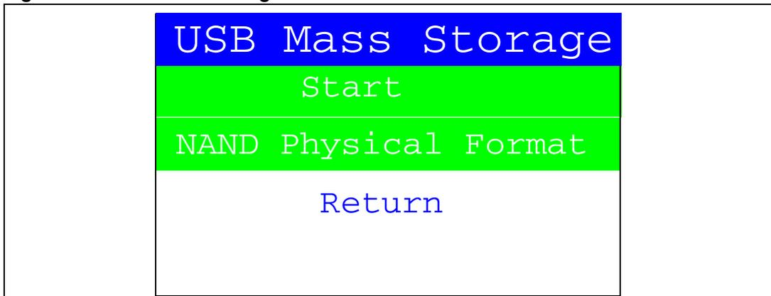
If the SEL push-button is pressed when Start is selected, the message shown in [Figure 43](#) appears on the LCD screen until the cable is plugged in.
