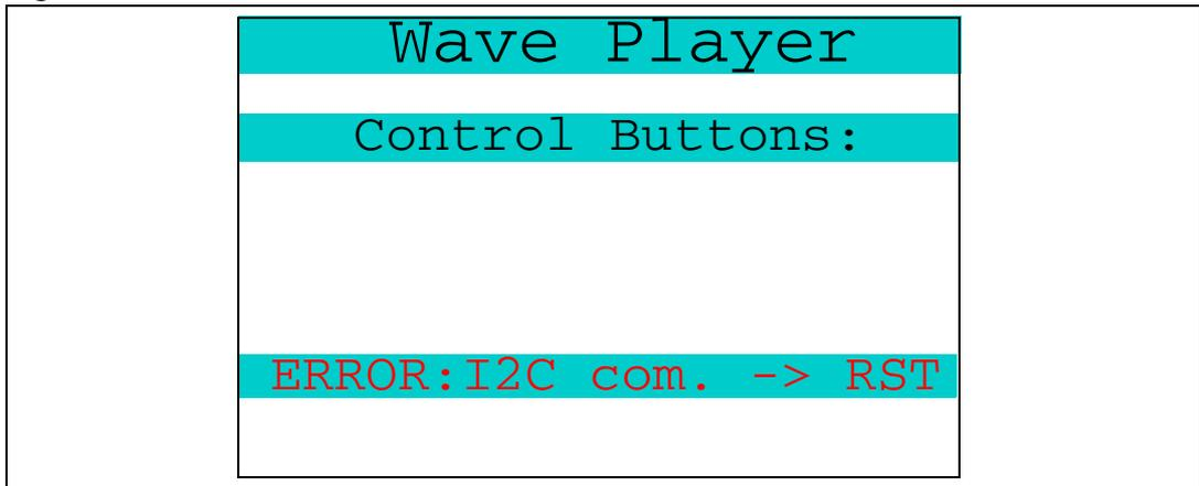
If the audio file is missing or if its format is not supported, the error message shown in *Figure 41* is displayed and a reset is required.
